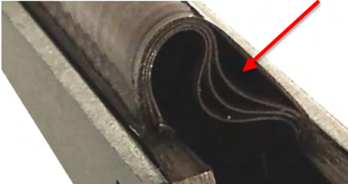
Fig. 3: In this commercially produced design, the designers obviously did not apply “bookbinder construction”, resulting in additional stress on the separated layers (red arrow). 7
